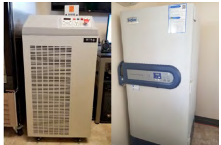
Left: Chiller for sub-zero perfusion | Right: "Dry ice" temperature freezer
